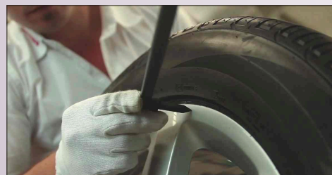
Automatic rim width measurement.
