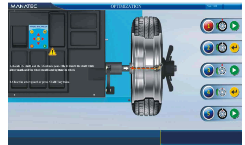
Optimization program helps in reducing wheel weight consumption.
