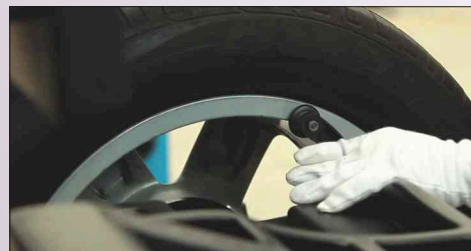
Automatic distance & rim diameter input through distance measuring rod.
